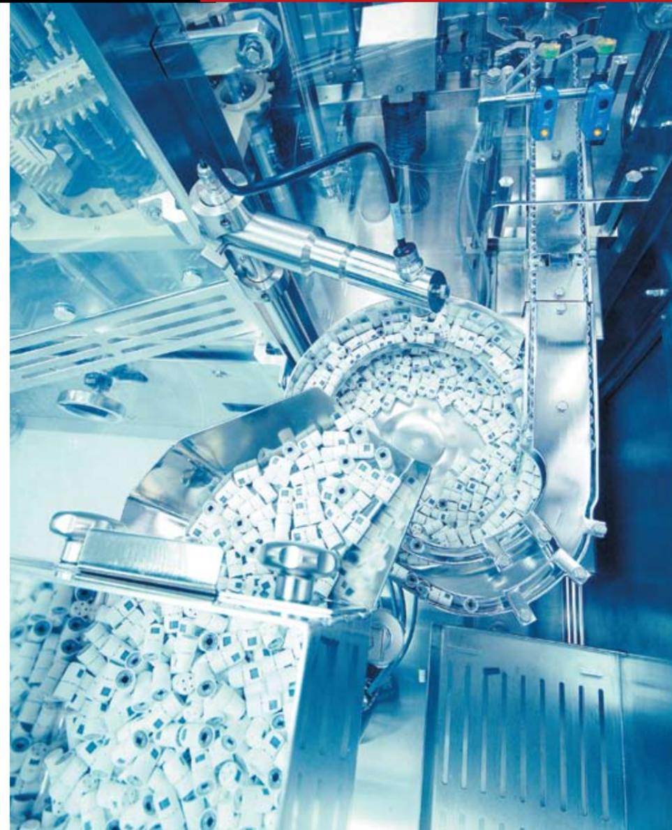
Processing of tamper-evident V-OVS® caps for bulk syringes.
