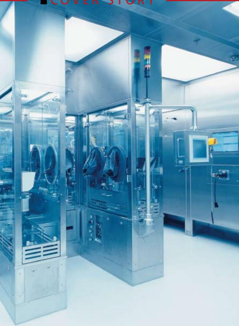
Above: Glove ports for the syringe line are integrated into the clean room wall; the human machine interface (HMI) displays process and environmental data for operators inside the clean room.
