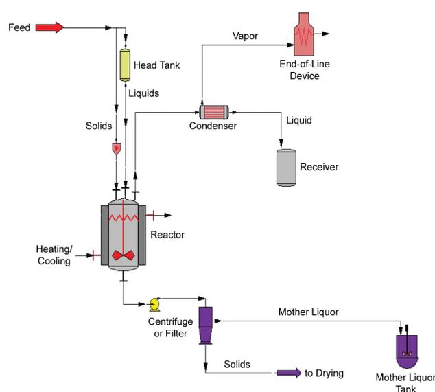
Figure 1. A Typical batch “single reactor” process train.
